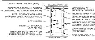
LOT GRADES AT PROPERTY CORNERS FRONT SETBACK = 4.0m LEFT LOT GRADE AT SHARED PROPERTY LINE AT GRADE CHANGE INTERIOR SIDE SETBACK = 1.3m EXTERIOR SIDE SETBACK = 4.0m LOT WITH FILL IN EXCESS OF 1.2m
